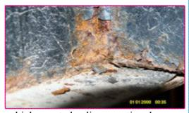
vehicle created a disproportional weight condition. Generally the cause is a corroded frame that has lost some of its structural strength, or it has been subjected to greater loads than it can now carry. Only in rare occasions have wire coat hanger will fracture from the the manufacturers been responsible for frames with multiple slide-outs were most prevalent.
